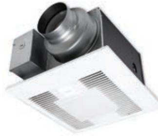
**(Energy) Star Products.** Panasonic's *WhisperGreen* Ventilation Fan combines a highly efficient motor, "smart" sensors and LED light to create an ultra-efficient and quiet fan/light combo. A condensation sensor tells the fan to turn on once the relative humidity exceeds a threshold, and a motion sensor activates the fan when someone enters the room.
