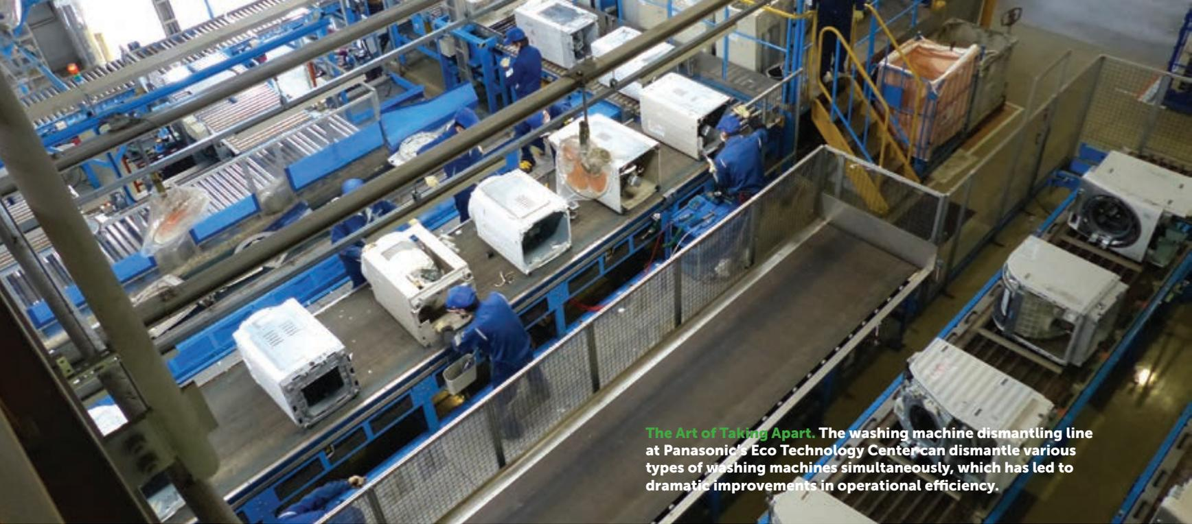
**The Art of Taking Apart.** The washing machine dismantling line at Panasonic's Eco Technology Center can dismantle various types of washing machines simultaneously, which has led to dramatic improvements in operational efficiency.
